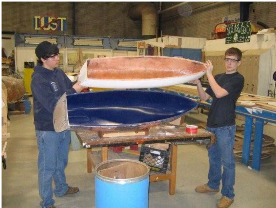
Hull #1 as she emerges from the master mold on March 9 th at the Mid-Coast School of Technology in Rockland, Maine
